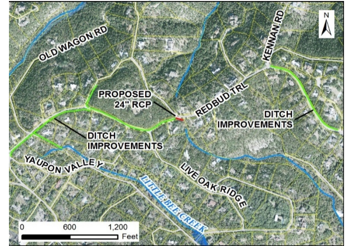
Proposed cross drainage and ditch improvements
