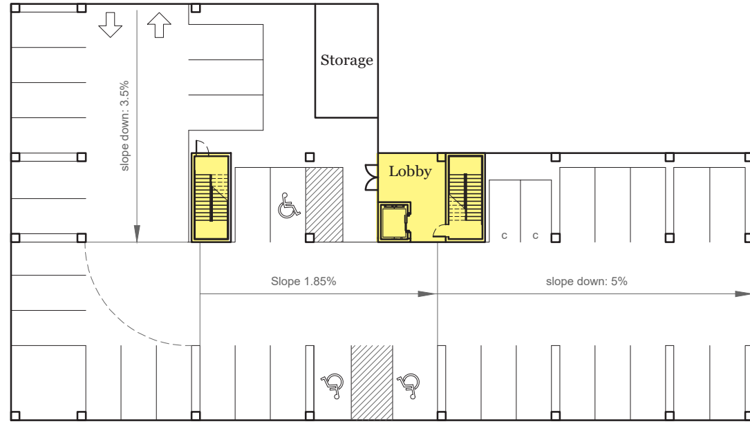
Garage Level 1 Floor Plan 1/32" = 1' 0"
