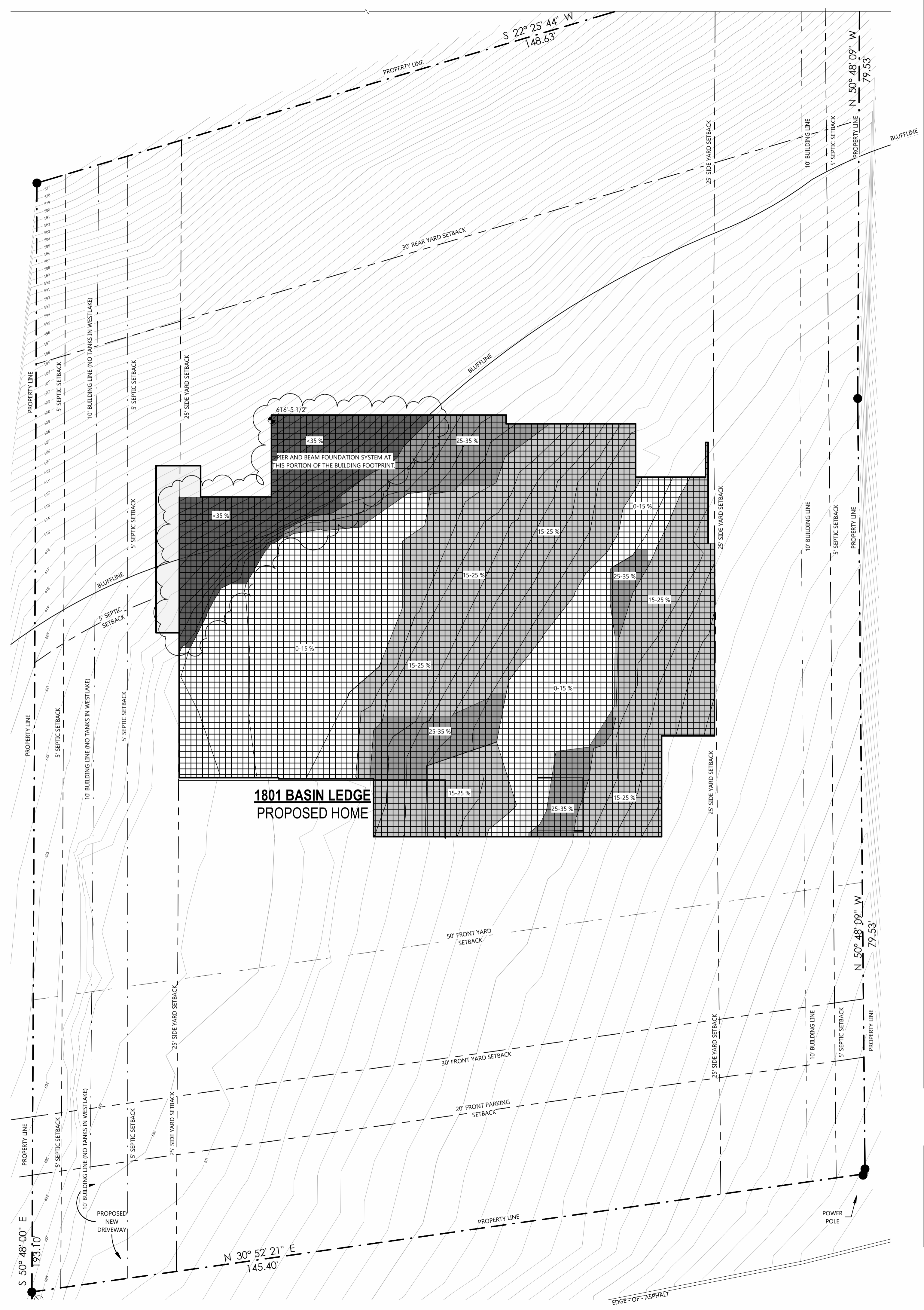
1 EXISTING SITE SLOPE ANALYSIS 1" = 10'-0"
