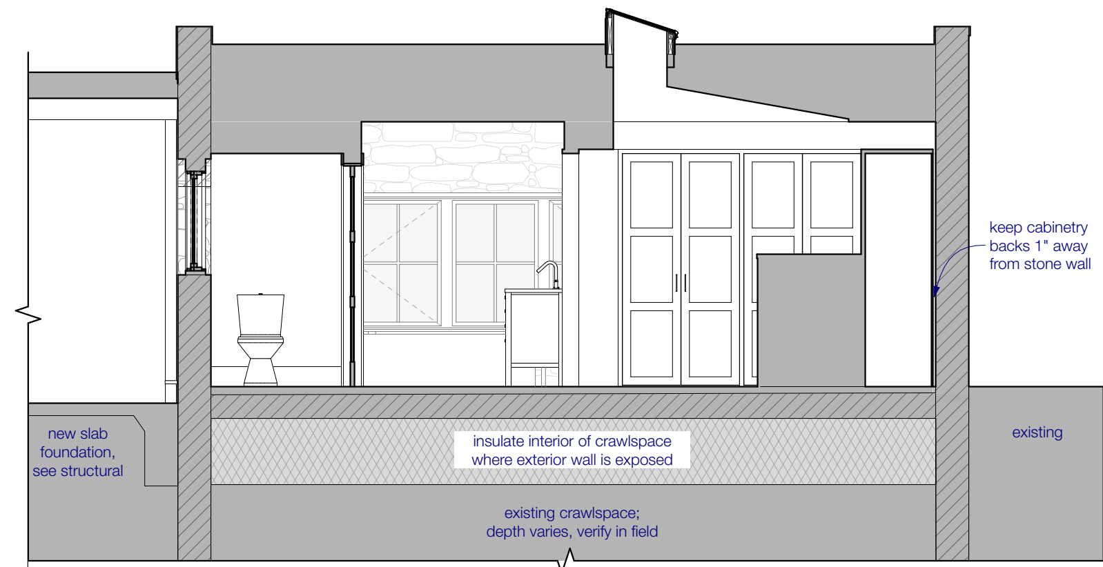
1 section @ master bath and closet SCALE: 1/4" = 1'-0"
